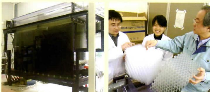
iPMBR reactor (left: anoxic tank, right: inclined plates)
